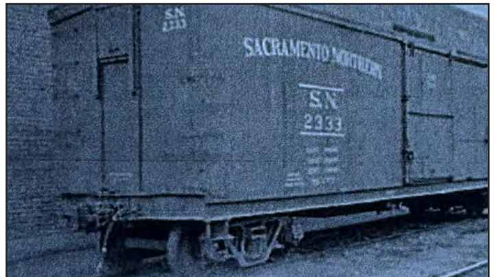
SAC Northern wood cars document photograph SN 2333 is shown here with wooden ends which were once common on this class boxcar.
