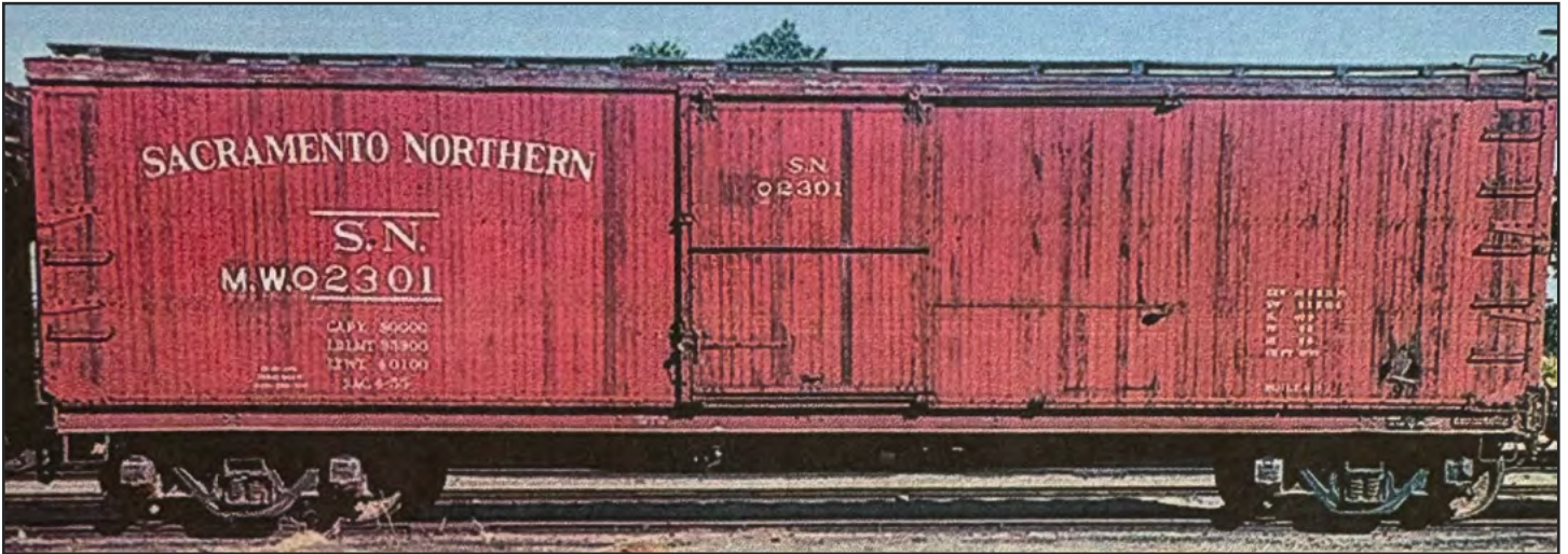
SN 2301 was the first car to be received from WP. The car was the only one with Murphy-ends. The rest of the 28 new cars starting with SN 2302 had Dreadnought ends.
