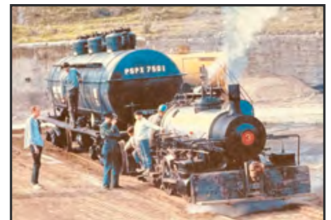
Tank car PSPX 7501 providing the necessities to steam up the new No. 3 at Castro Point Railway.
